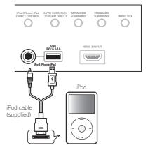
• Switch the receiver into standby then use the supplied iPod cable to connect your iPod to the iPod iPhone iPad USB terminal on the front panel of this receiver.
